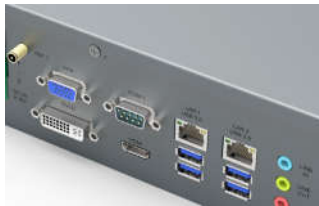
Side B - Huge I/F capability towards the field, 3 display ports , 4 USB 3.0 , 2 independent LAN ports.
